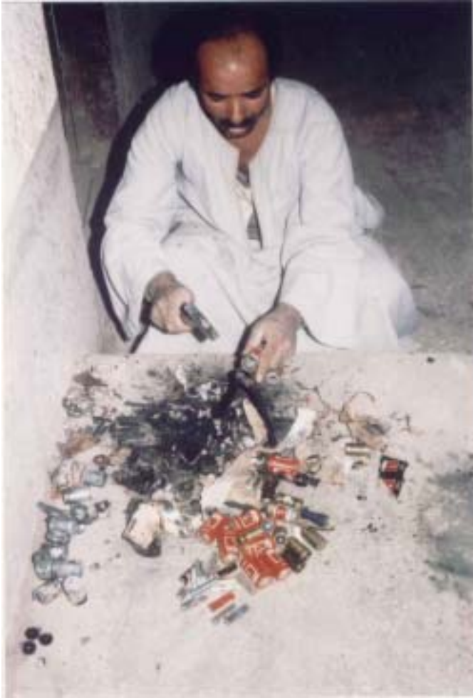
Picture 1 and 2 Dismantling of household batteries in Cairo, Egypt.
